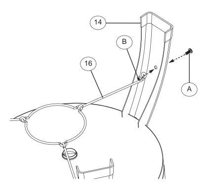
Attach drip cup holder (16) to leg (14) using pan head screw (A) and hex nut (B) as shown.
